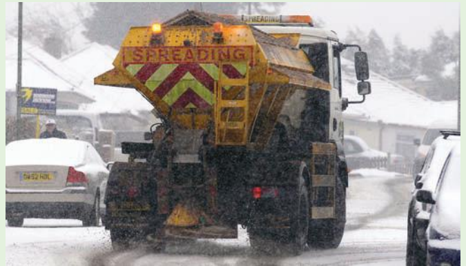
Figure 3.17 Salt gritter at work to prevent ice formation on a road
